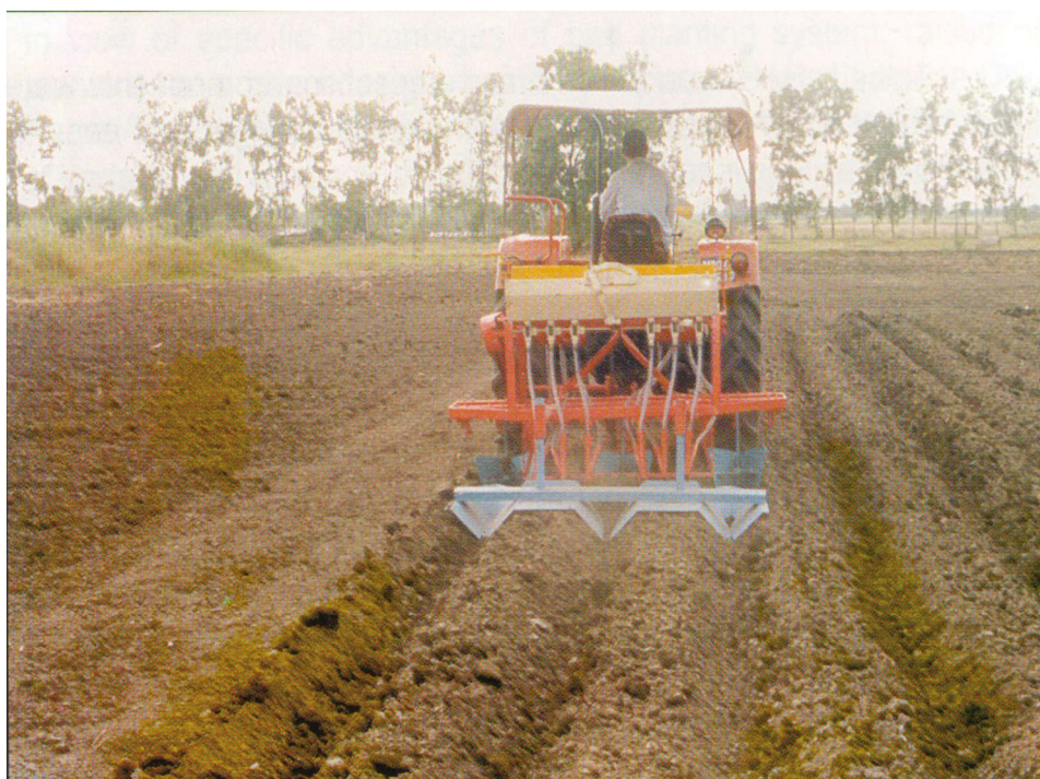
Fig. 7.1: Field operation of raised bed planter for bed planting of wheat.
