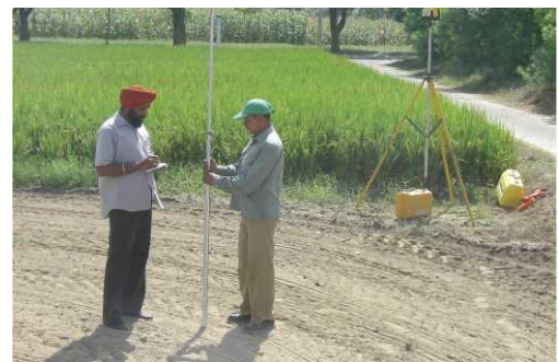
Fig. 8.1: Field adjustment of laser emitter.
