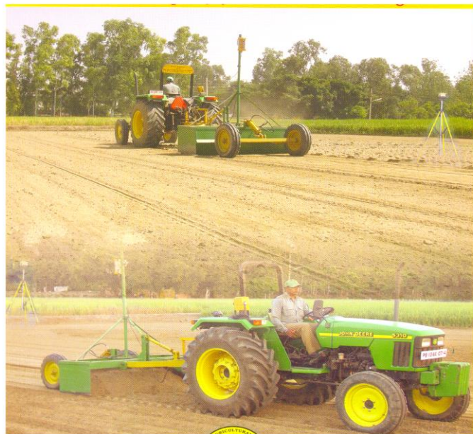
Fig. 8.4: Tractor operated laser land leveller leveling field.
