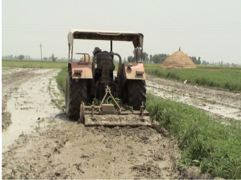
Fig. 1.4: Tractor operated rotavator incorporating Dhaincha (green manuring & puddling simultaneously) in standing water for paddy cultivation.
