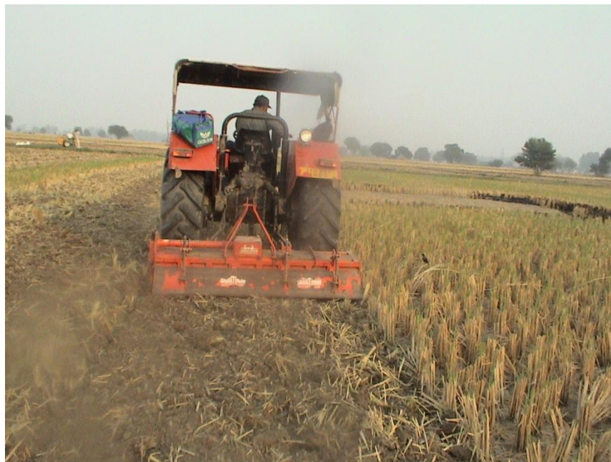
Fig. 1.5: Tractor operated rotavator used to prepare seed bed in single operation after harvest of paddy crop for sowing wheat crop.
