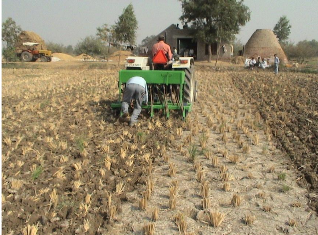
Fig. 3.3: Zero-till seed-cum-fertilizer drill in operation in paddy harvested field.
