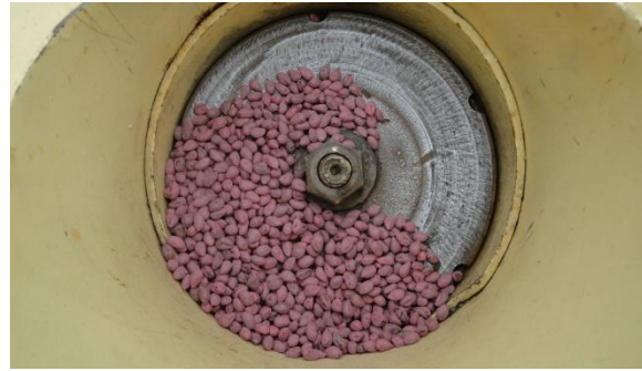
Fig. 4.1: A view of Bt. Cotton planter Fig. 4.2: View of inclined plate with cells
