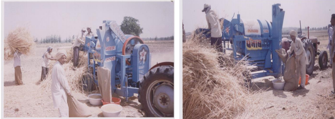
Fig. 7.2: A view of operation of high capacity multicrop thresher on custom hiring in wheat crop at farmer's fields.
