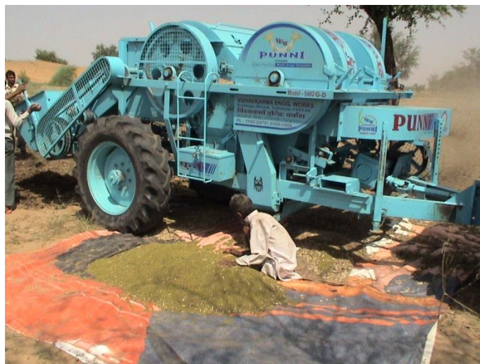
Fig. 7.4: Threshing green gram crop with high capacity front feeding thresher on custom hiring.
