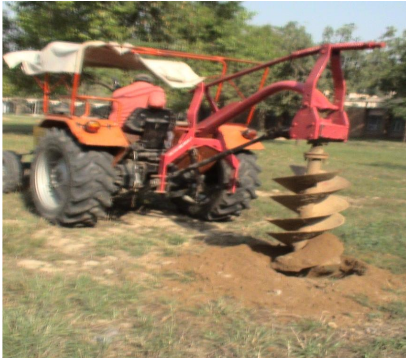
Fig. 10.1: A view of post hole digger in operation at farmer's fields.
