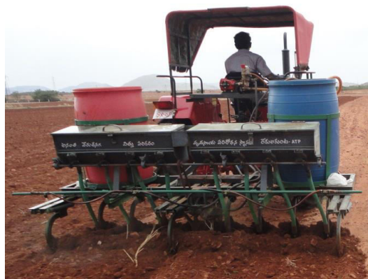
Fig. 1. Testing of planter cum boom Sprayer for groundnut crop.
