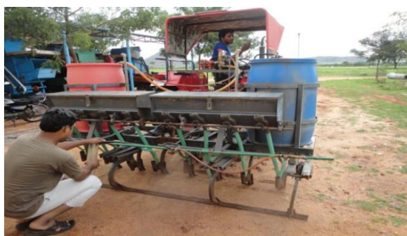
Fig. 3. Calibration of the nozzle rate
