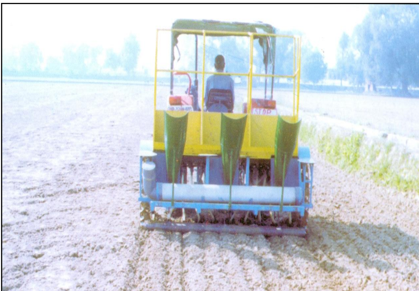
Fig. 2. IISR Multipurpose planter in operation (Seed drill mode)
