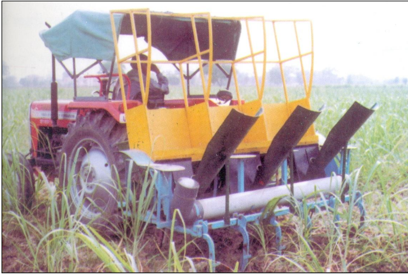
Fig.1 IISR Multipurpose planter in operation (Interculture mode)
