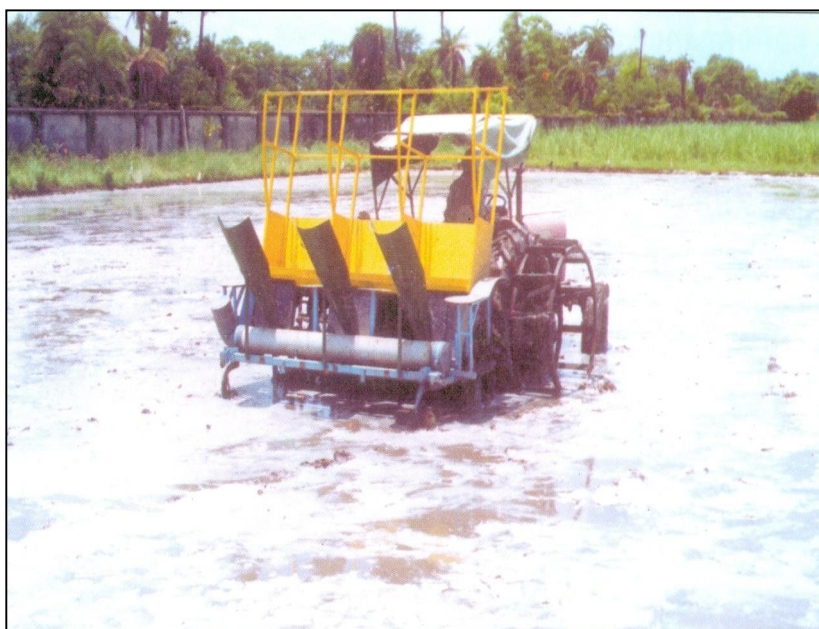
Fig. 3 IISR Multipurpose planter in operation (Puddler mode)
