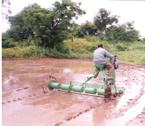
Fig. 1. Self-propelled 10 row paddy seeder.
