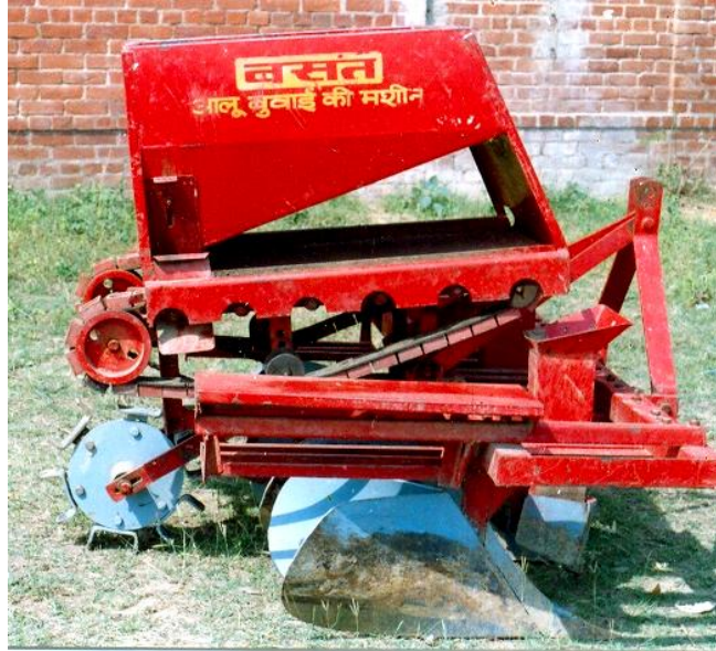
Fig. 1. Semi - automatic potato planter
