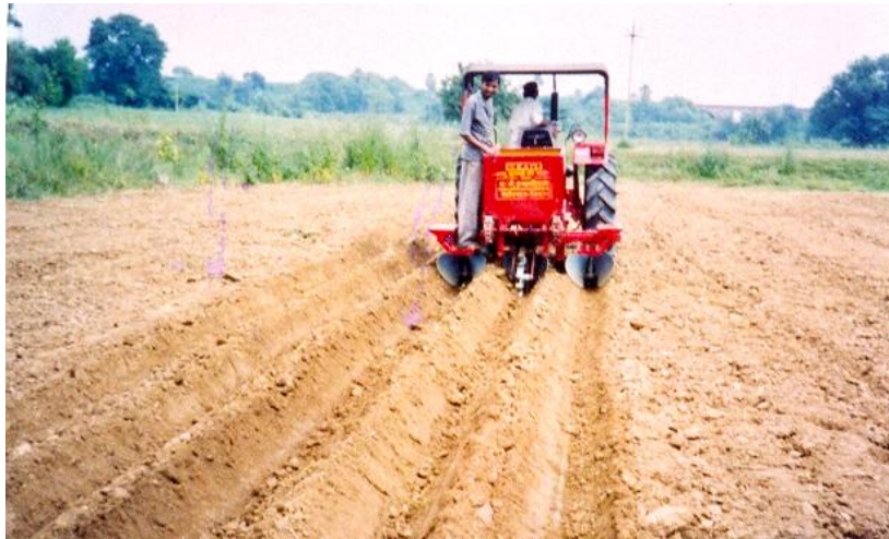
Fig. 2. Semi-automatic potato planter in operation
