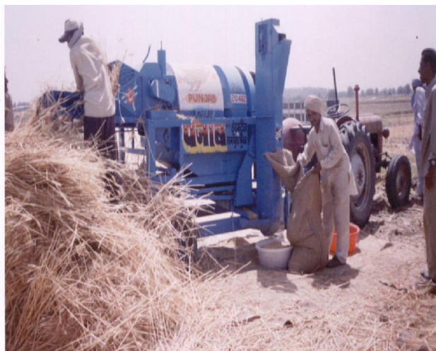
Fig. 1. High capacity multicrop thresher on custom hiring in wheat crop at farmer's fields.
