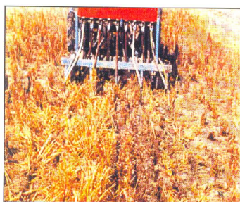
Fig.1 Zero Till Seed cum Fertilizer Drill in operation for sowing wheat crop
