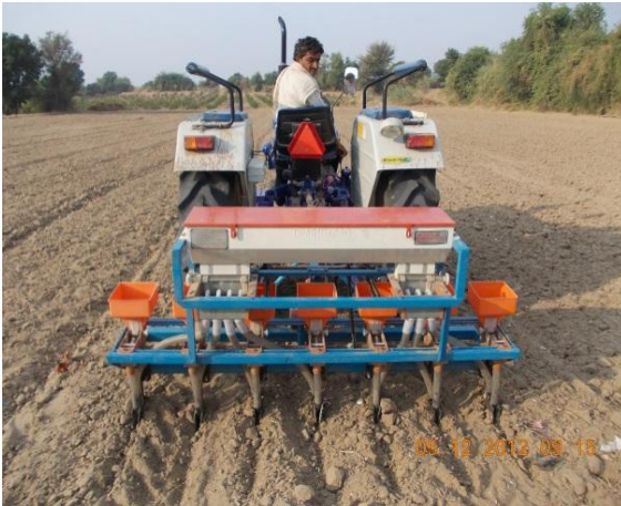
Fig. 1.3. Sowing of ajwain and cumin seeds by seed spices planter.
