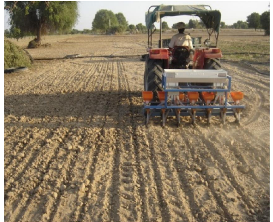
Fig. 1.3. Sowing of ajwain and cumin seeds by seed spices planter.
