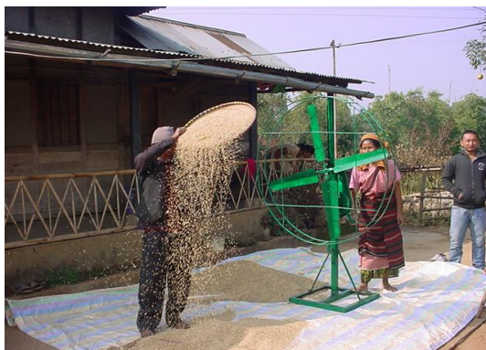
Fig. 4.3. Cleaning of paddy by a farmer of Meghalaya using hand operated winnower.
