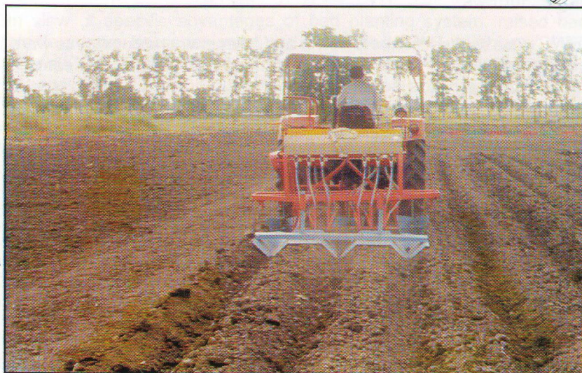
Fig 1 Field operation of raised bed planter for bed planting of wheat
