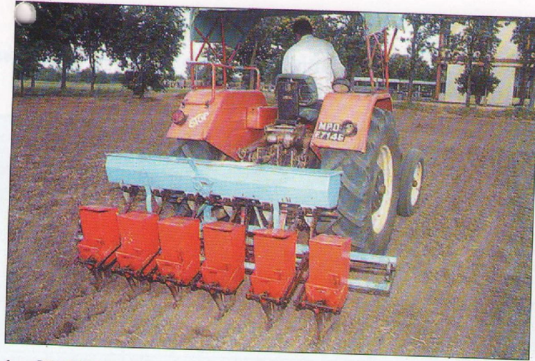
Fig.1: CIAE Tractor mounted inclined plate planter with fertilizer box
