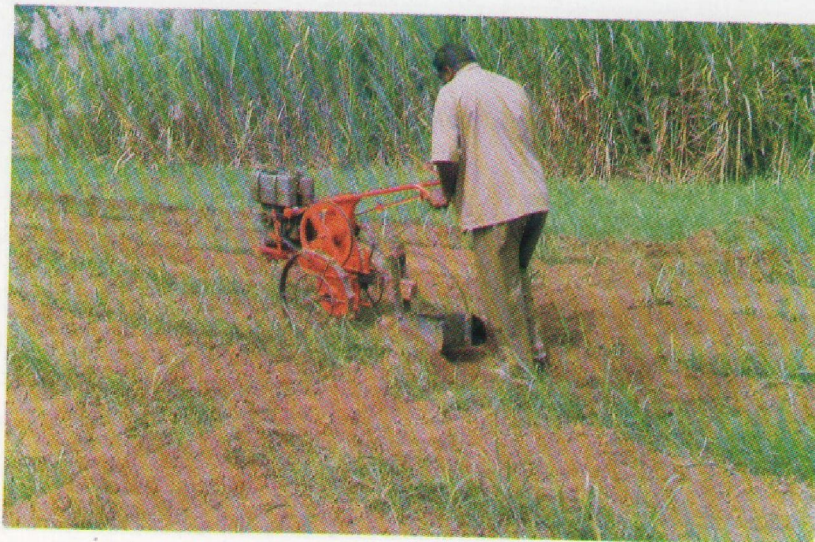
Fig. 3: Power Weeder with Ridger Attachment in Sugarcane Field
