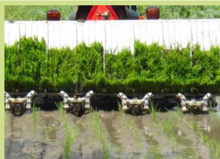
Fig. 2 Demonstration of 4-wheel drive tractor mounted 8-row paddy transplanter at farmer's field.
