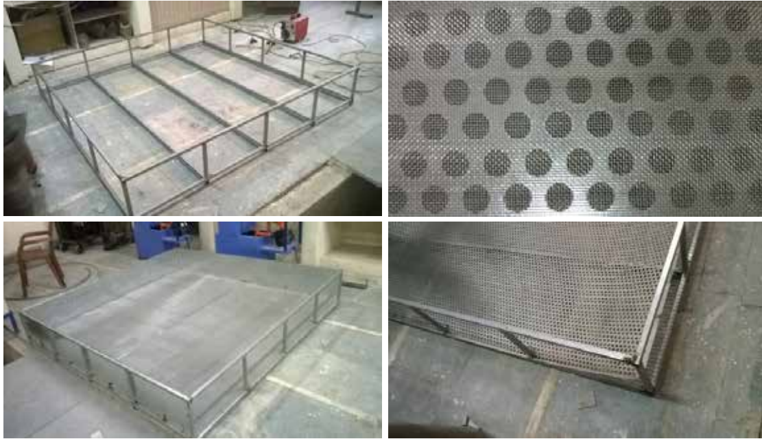
Fig. 4.1.1. Bottom, top and side view of construction details of screen gravel filter
