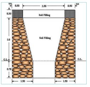
skill. A cross-sectional view of the low cost dry stone masonry structure is shown in the figure.
