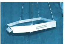
is sieved. The overall dimension of the equipment is 900x600x140 mm and weight is 17.6 kg. The machine has top (5-8.5 mm diameter sieve) and bottom screens (18x20 mm to 32x20 mm) that can be changed according to the requirement of the grain to be cleaned. The machine gives cleaning efficiency in the range of 99.0-99.8%. Its operating cost is Rs. 5.3/q.
