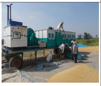
moisture laden air at the top drying chamber. Intermittent tempering of the grain during /after drying equalizes the moisture distribution within the grain and aid in uniform drying. Dried grains can be discharged through gravity outlets provided.
