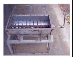
shaft in zigzag manner for facilitating scrapping of hot thick jaggery syrup into crystal/crystal form. Crystal jaggery making machine further modified by keeping rectangular projections (of 30 mm width and 32 mm length) with sharp edges at the end of the blades and were welded for easy shearing of jaggery into crystal form. This machine is superior in terms of saving time and drudgery.
