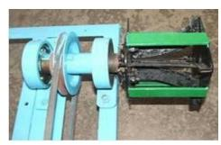
mounted on a rectangular frame. The unit is operated by electric motor(1 h.p.) through belt and pulley arrangement.
