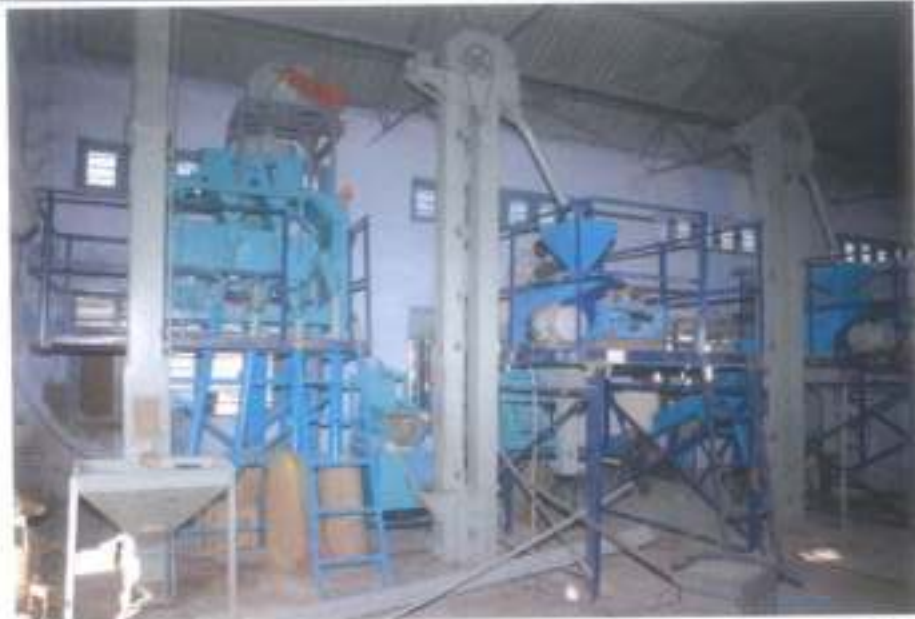
DAL MILL PLANT (0.5 t/h) BASED ON CIAE MINI MILL DESIGN (Bhopal centre)
