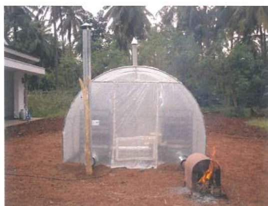
Solar Tunnel Dryer with Biomass backup Heater for Cocoa Beans Drying (Coimbatore)
