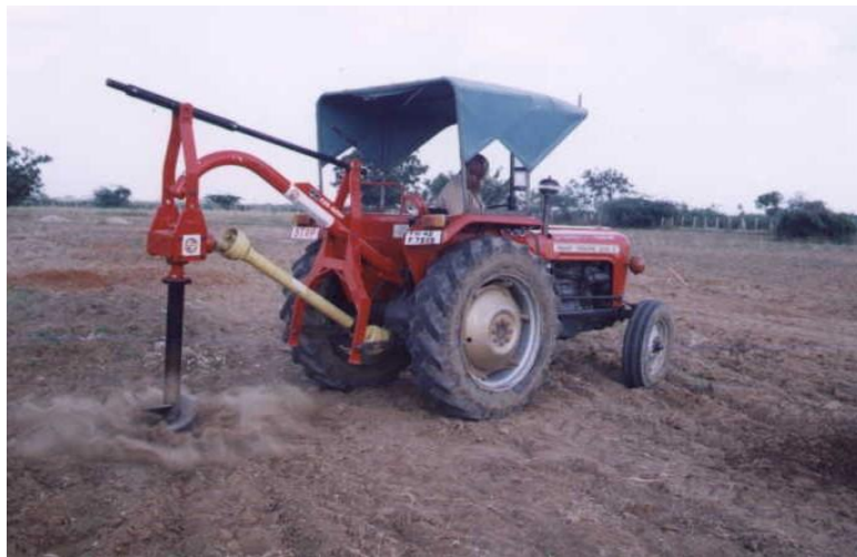
Plate 4. Planting technique using Auger hole
