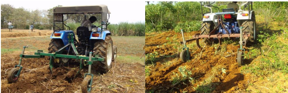
Fig. 4. Operation of single row and two row Cassava harvester in field.
